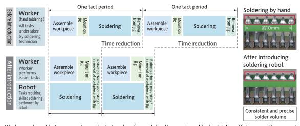
Works are shared between worker and robot and performed simultaneously, achieving higher efficiency and lower cost No reliance on individual soldering skills brings improved soldering quality
